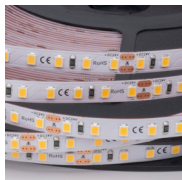
24V 25mm cut 13W/m Ra90+ 120LED/m
