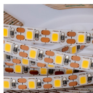
12V 8.33mm cut 10W/m Ra90+ 120LED/m
