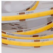
12V 25mm cut 12W/m Ra90+ 480LED/m Dotless
