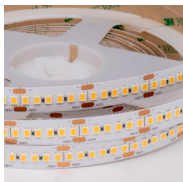
24V 25mm cut 19.5W/m Ra90+ 240LED/m Dotless
