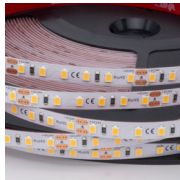
24V 50mm cut 13W/m*2line Ra90+ 240LED/m Dotless
